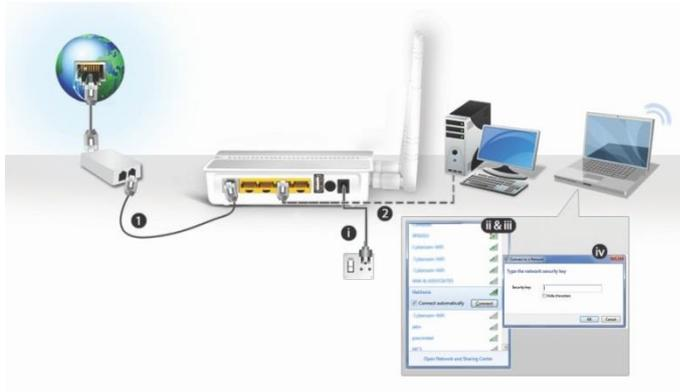
This shows connecting the NetGenie via splitter or ADSL filter. Which is not typically required. You can plug the supplied RJ11 ADSL/VDSL cable directly into your telephone master socket, where the ADSL/VDSL socket is located. Plug the other end of the cable into your NetGenie.
